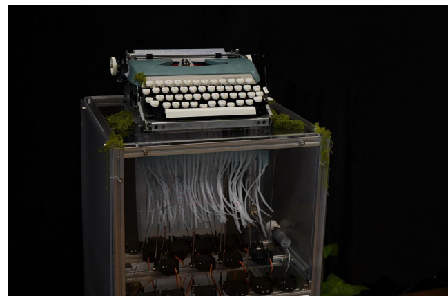
Figure 4. Type & Fade installation overview, featuring a servo-driven vintage typewriter and an integrated paper-shredding mechanism.
