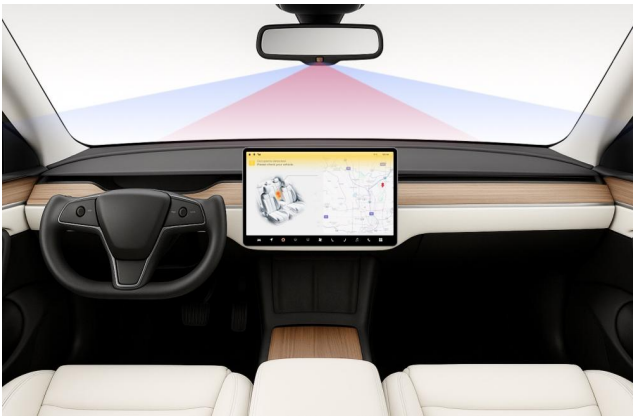
Figure 1. Thermal Sense system overview, combining the in-cabin UI display with a rearview mirror-embedded thermal sensing module.
